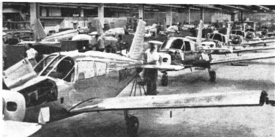
Above, Piper Cherokees on the production line at Vero Beach, Florida. Current production rate of the type, which sells for £5,200 in Britain, exceeds three per day
